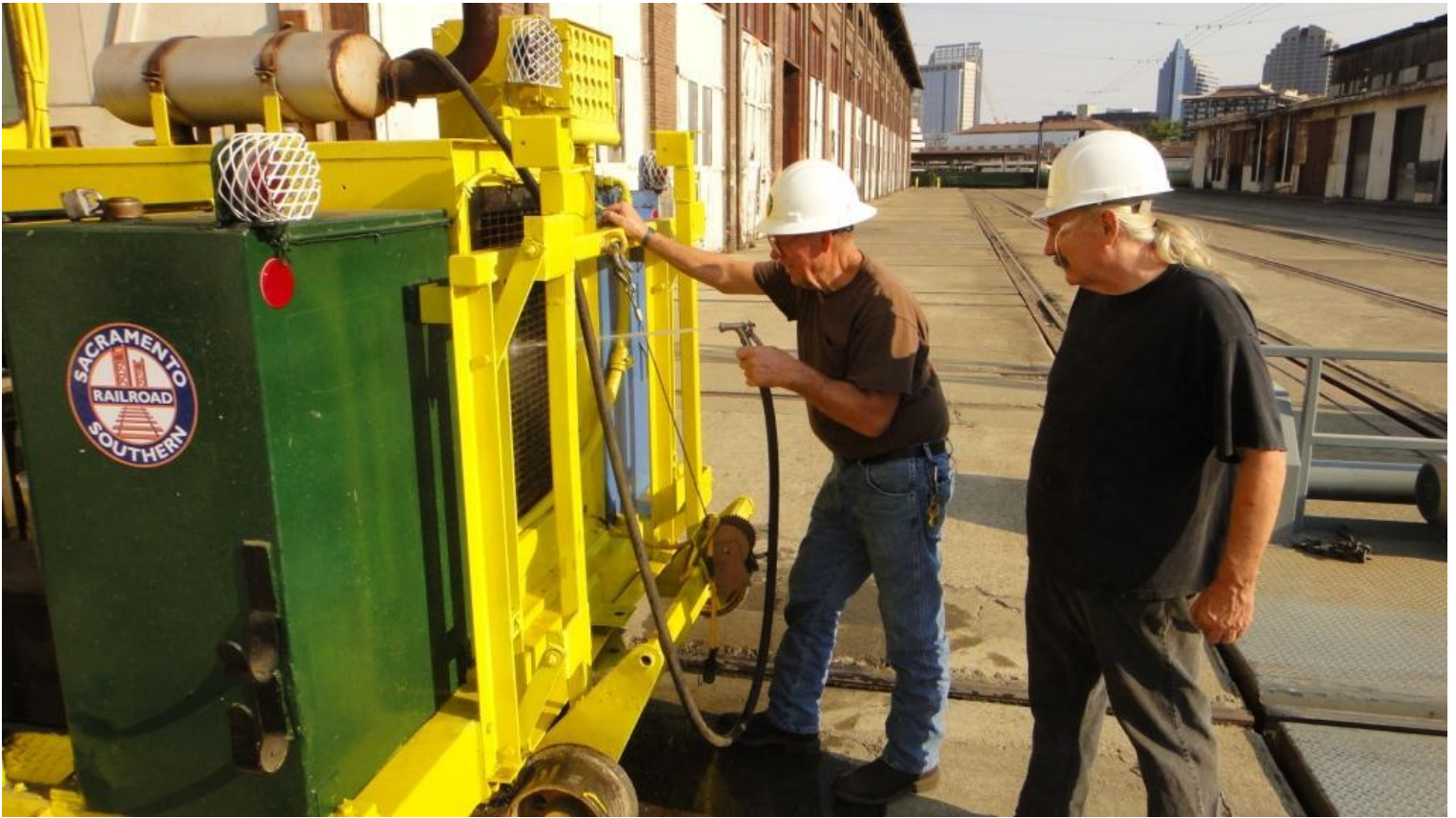
Cliff and Fred clean out the radiator of the tamper
